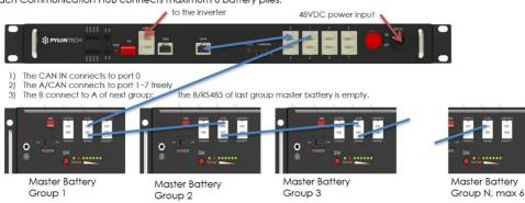
Each battery pile can configure maximum 16pcs US2000C/US3000C.
